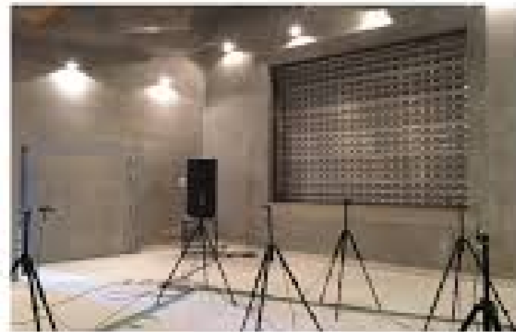
Receiving room (RCI)
